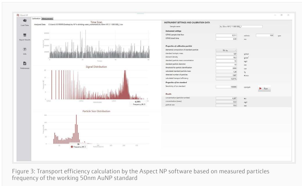
Figure 3: Transport efficiency calculation by the Aspect NP software based on measured particles frequency of the working 50nm AuNP standard
