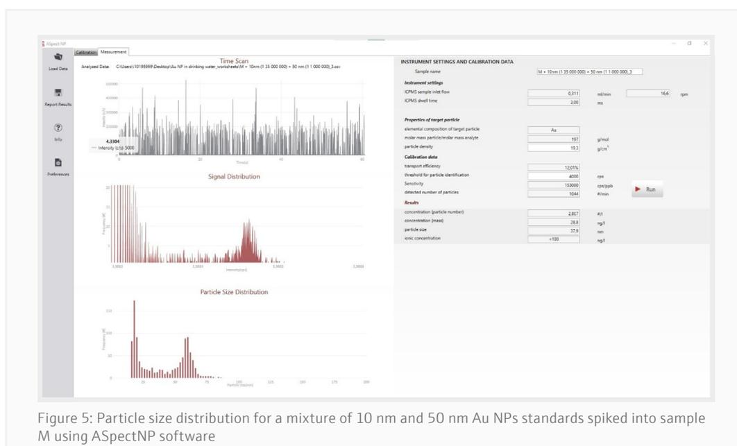
Figure 5: Particle size distribution for a mixture of 10 nm and 50 nm Au NPs standards spiked into sample M using ASpectNP software
