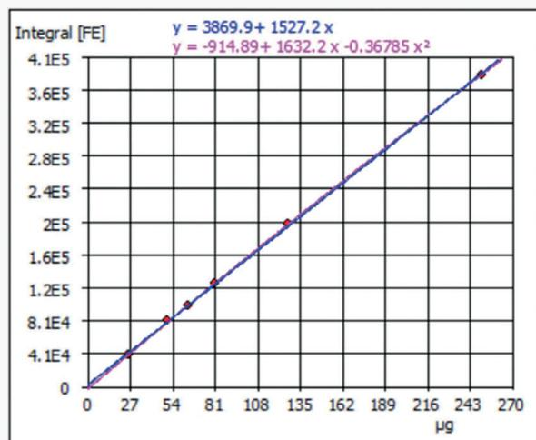
Figure 2: Example of a calibration curve TIC 50–500 mg/L
