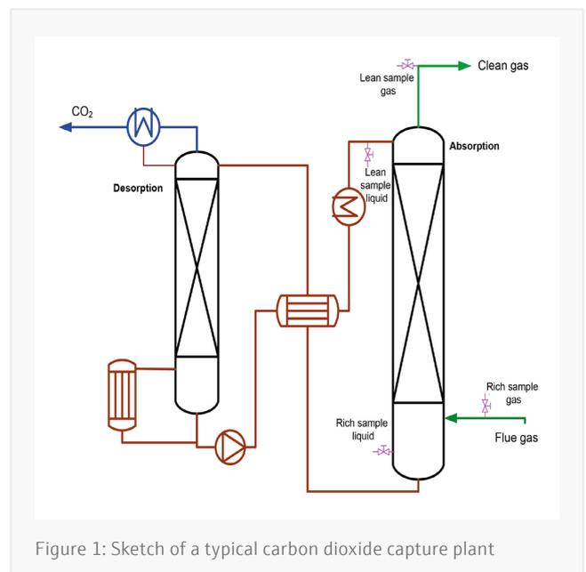
Figure 1: Sketch of a typical carbon dioxide capture plant
