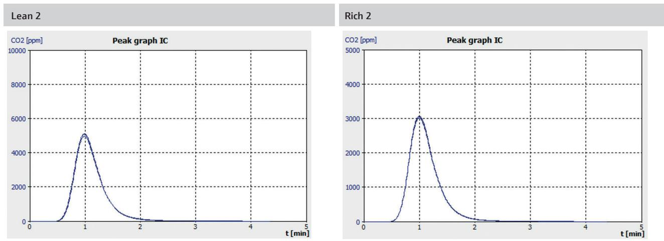
The example measurement curves illustrate the excellent reproducibility of the measured values within a multiple injection from a sample vessel. As a result, the TIC method shows the lowest deviation to the known amount of added CO<sub>2</sub> and also the lowest standard deviation in comparison of the analysis methods.
