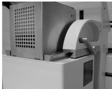
Fig. 23: Take off the pipetting head
