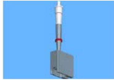
2. Slowly slide one of the threaded O-rings along the O-ring guide pin toward the cone until it reaches its groove.
