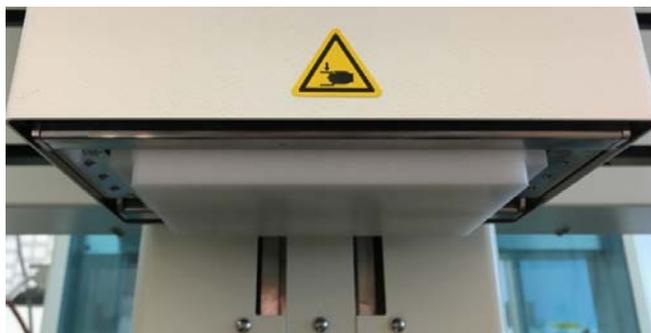
Fig. 46: Cover magazine (transport protection) attached
