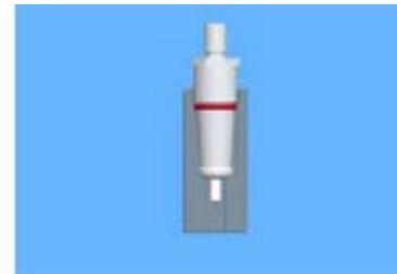
2. If this attempt at O-ring removal was unsuccessful, there is still an alternative solution for removing the O-ring. To do this, turn the O-ring assembly tool around. There is a tip here (on the side of the O-ring guide pin) that can also be used to remove the O-ring. For this purpose, press the tip against the O-ring and then remove it.
