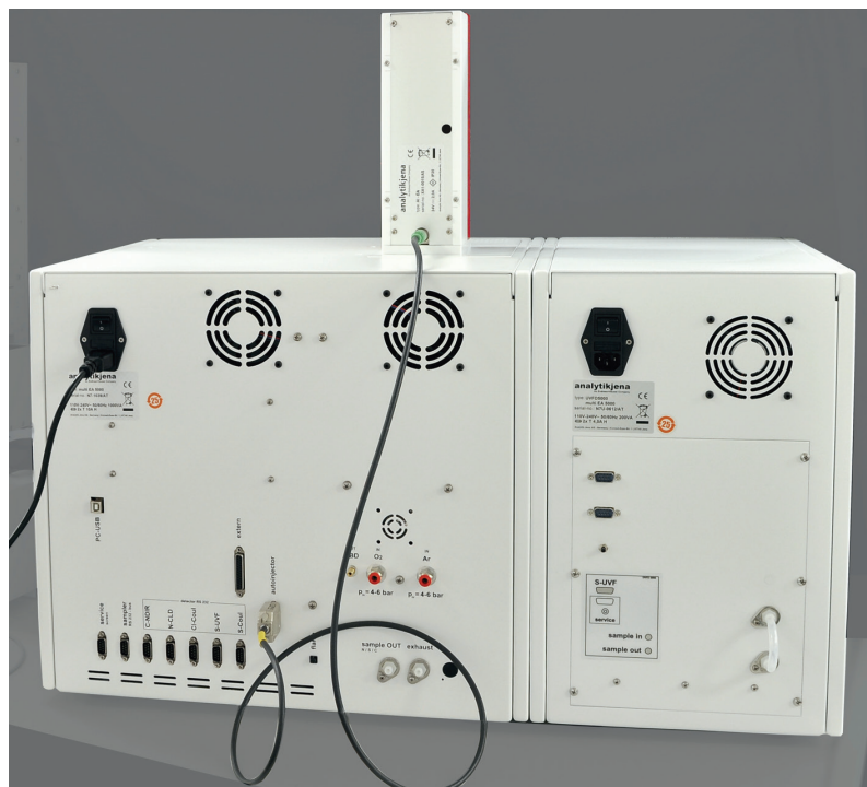
Fig. 5 Autoinjector connection to the elemental analyzer
