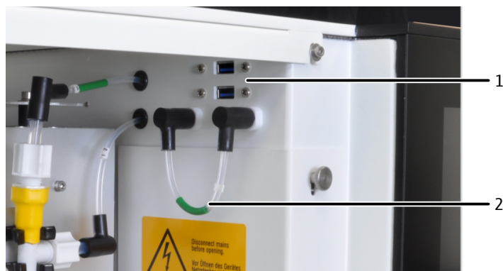
Fig. 18 USB ports and hose bridge in the gas path behind the front door
