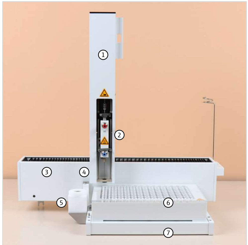
Fig. 2 Main components of the autosampler
