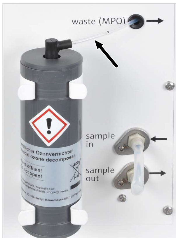
Fig. 73 Replacing the chemical ozone decomposer
