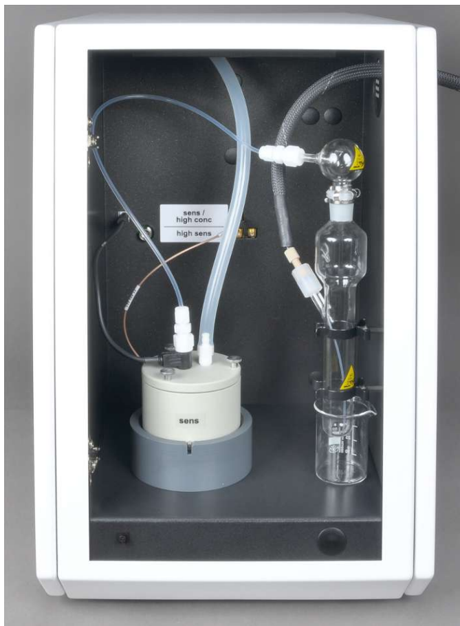
Fig. 40 Gas introduction into the "sensitive" measuring cell
