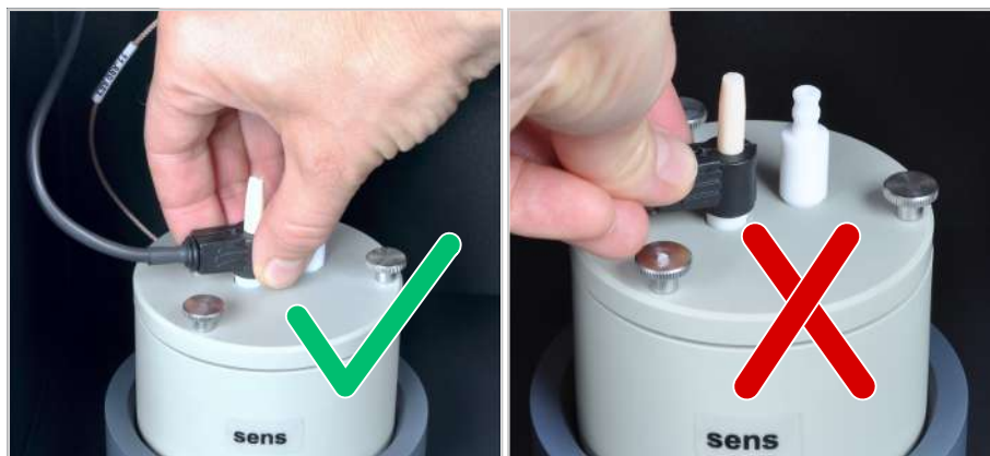
Fig. 72 Correct handling of the combined electrode
