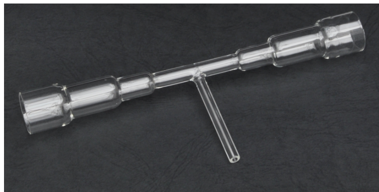
Fig. 11 Hg cell (made of quartz, tulip-shaped)
