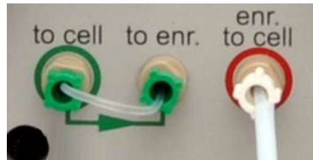
Fig. 18 Hose routing for the "Hg with enrichment" mode
