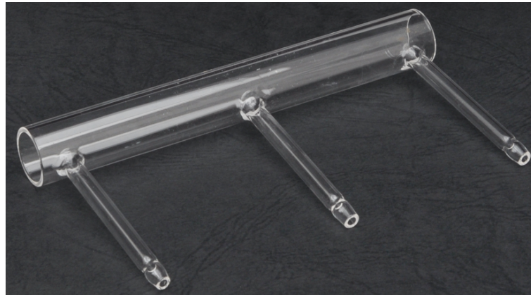
Fig. 10 Quartz cell for hydride method
