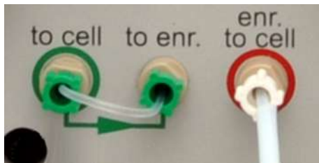
Fig. 20 Hose routing for the "Hg with enrichment" mode
