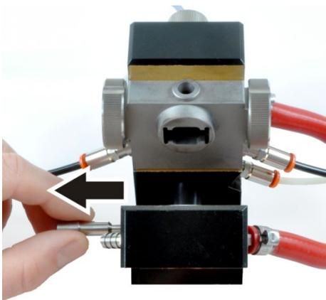
6. Pull out the lock pin for the movable furnace part and fold the movable furnace part all the way down.
