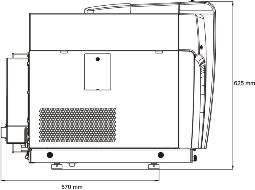
Fig. 4 contrAA 800 dimensions – side view
