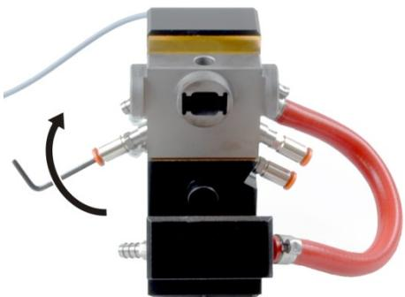
10. Remove the three gas hoses. To this end press in the quick-release lock and pull off the hose.
