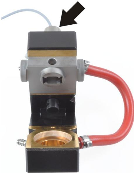
18. Screw the sensor sleeve for the cooling water temperature sensor carefully by hand into the fixed furnace part.
