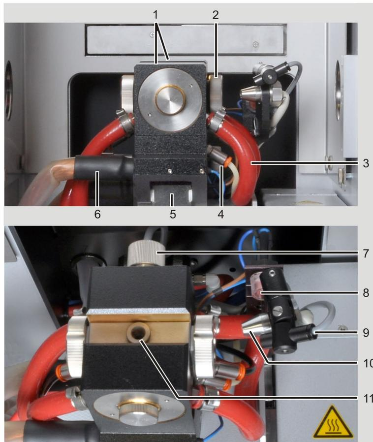
Fig. 12 Graphite tube furnace in the sample chamber
