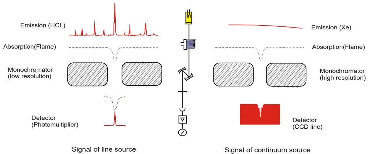
Fig. 7 principle of measurement of LS AAS and HR-CS AAS
