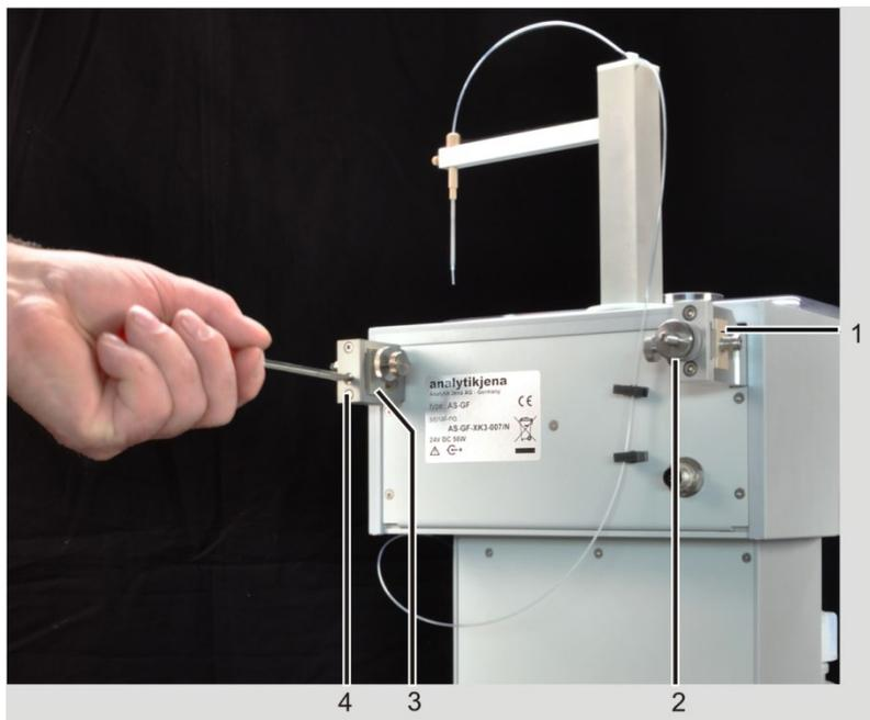
Fig. 38 AS-GF with screws for furnace alignment
