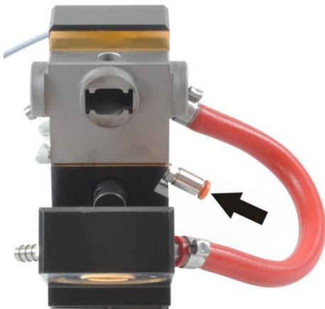
21. Screw the gas connectors for the outer gas flow transversely from below finger-tight into the fixed furnace part.
