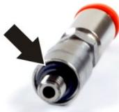
20. Check the sealing rings of all three gas connectors and replace if damaged.
