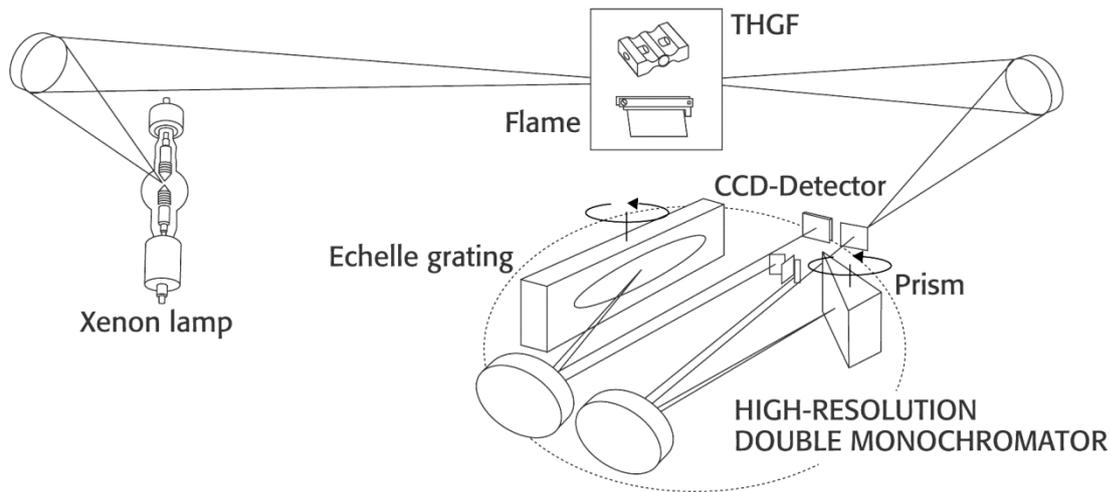
Fig. 10 Beam path in the contrAA 800
