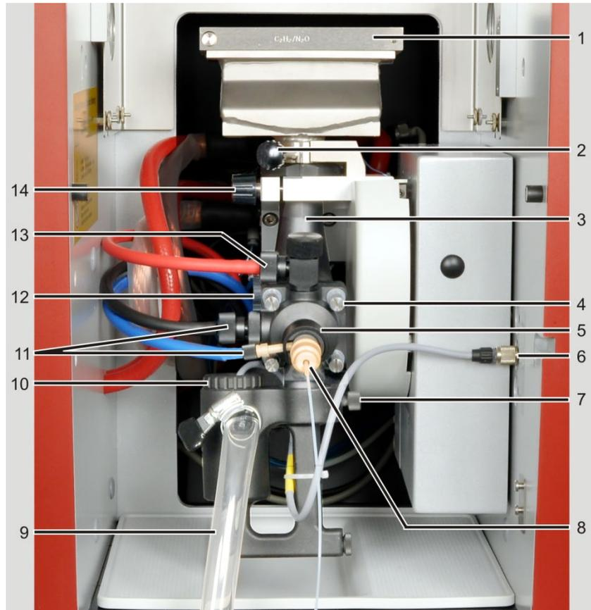
Fig. 54 Burner-nebulizer system
