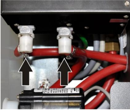
8. Connect the cooling water hoses at the underside of the lamp housing.
