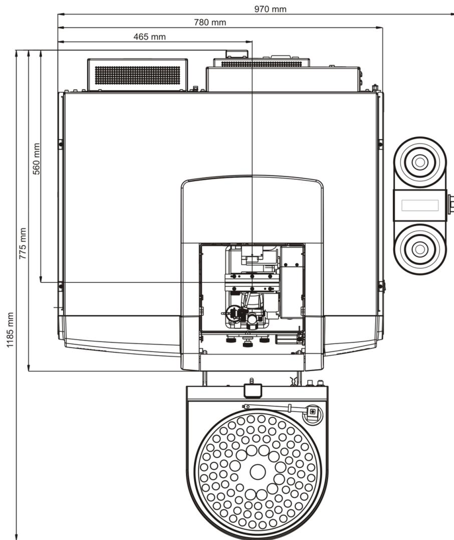
Fig. 5 contrAA 800 dimensions – top view (with autosampler AS-FD)
