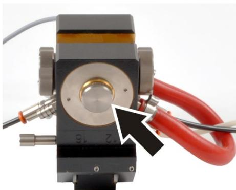
27. Screw the covering screw to the movable furnace part.
