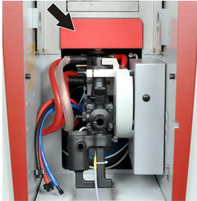
Fig. 31 Transport lock in the sample chamber of the contrAA 800 D
