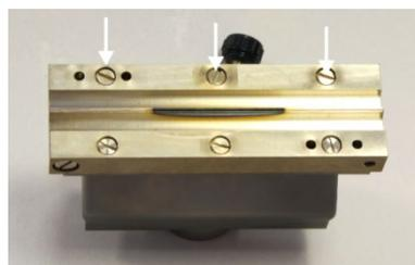
Fig. 47 Screws on the front burner jaw
