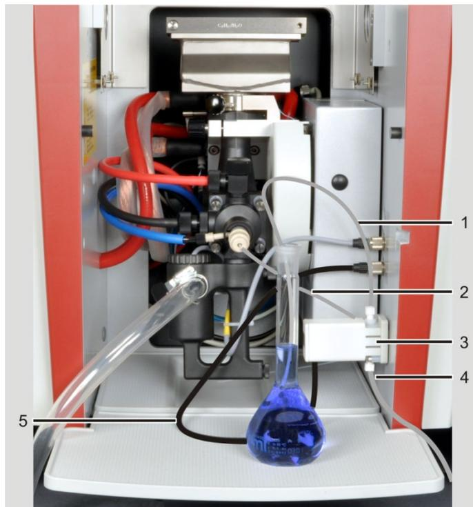
Fig. 46 Installing the SFS 6 for manual sample supply
