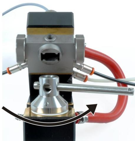
7. Release the insulating ring carefully with the pin wrench and unscrew it completely by hand.
