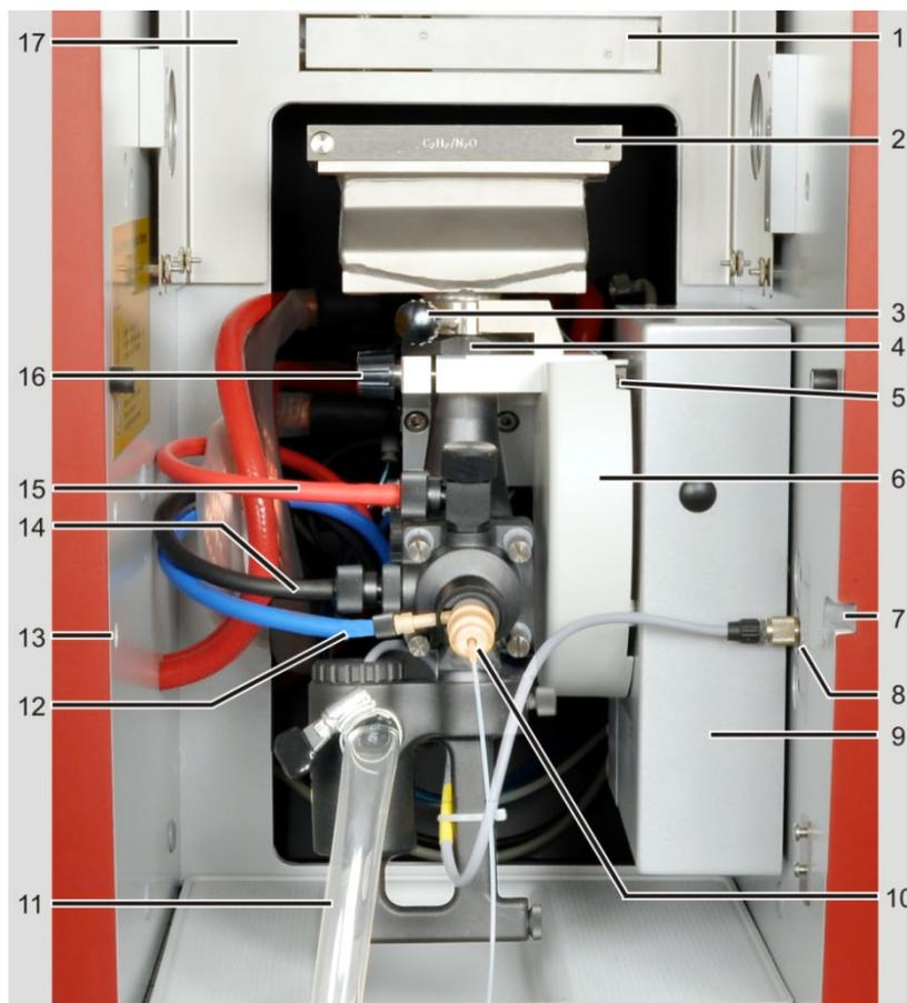
Fig. 41 Connections at the burner-nebulizer system
