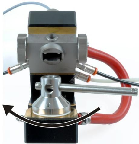
24. Attach the furnace windows to the furnace jacket. Insert the pipetter insert.
