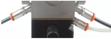
22. Screw the two other connectors (for the inner gas flow) on both sides into the furnace jacket.
