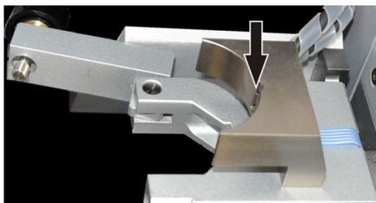
Fig. 59 Sensor openings for the burner detection
