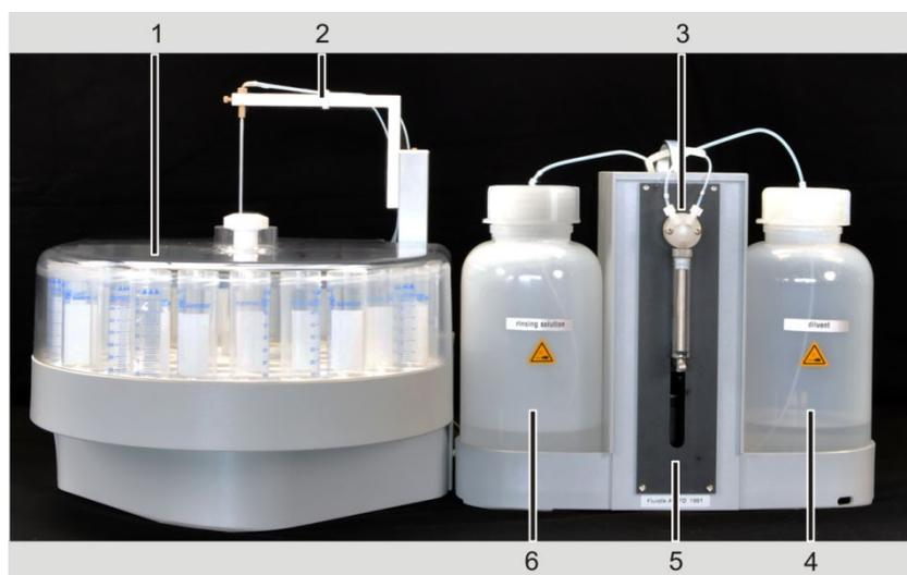
Fig. 23 Autosampler AS-FD with Fluidik module
