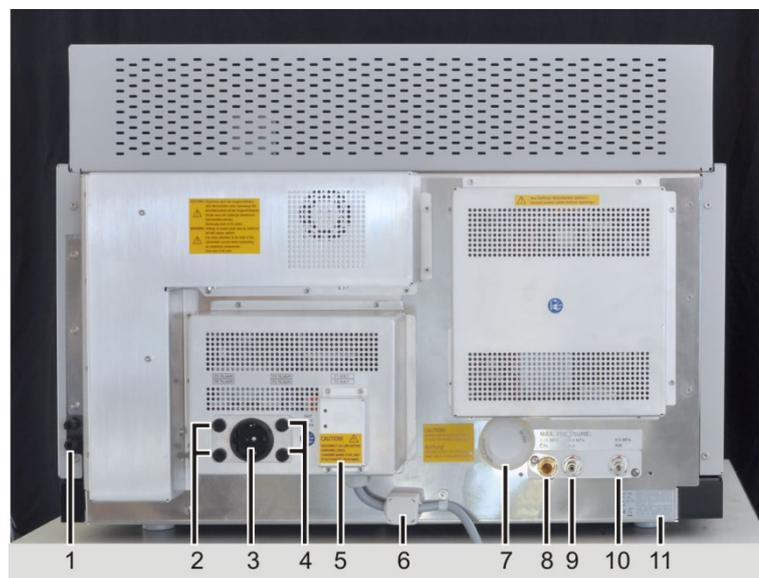
Fig. 27 Rear view contrAA 800 D with connections and fuses
