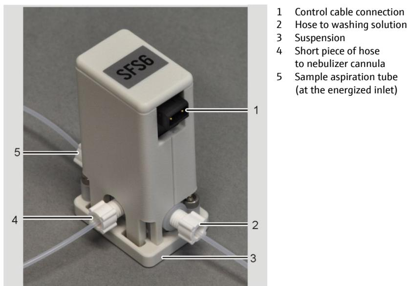
Fig. 24 Injection module SFS 6
