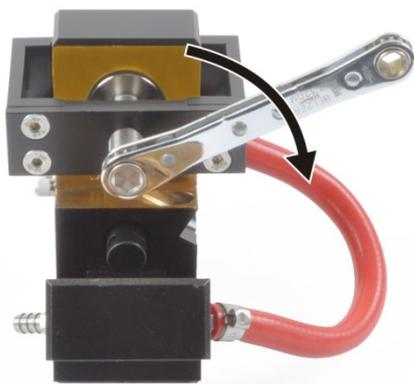
14. Position a new electrode parallel to the fixed furnace part and secure it with the inserting tool (small bracket).
