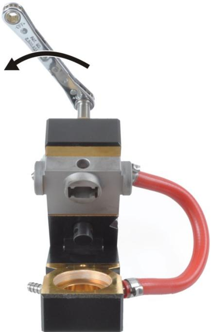
13. Screw the press-out tool with the spindle turned back to the stop into the fixed furnace part.
