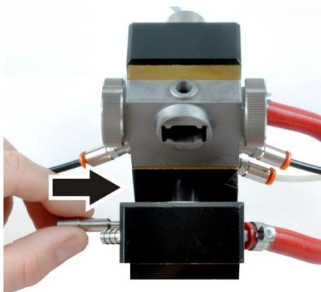
26. Insert the locking pin into the furnace jaw and connecting rod (arrow) up to the stop. The connecting rod must be in the front position.
