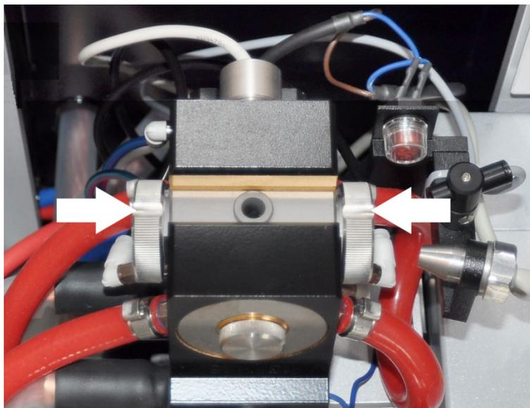
Fig. 51 Markings at the furnace windows
