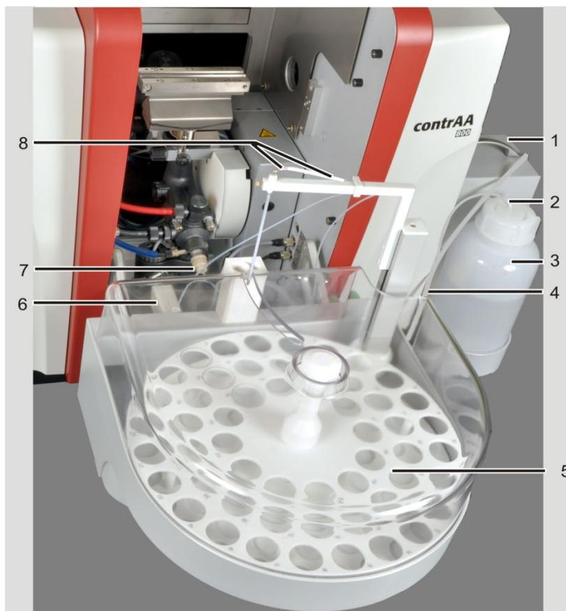
Fig. 43 Flame technique with autosampler AS-FD and SFS 6
