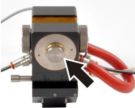
5. Unscrew the covering screw from the movable furnace part.
