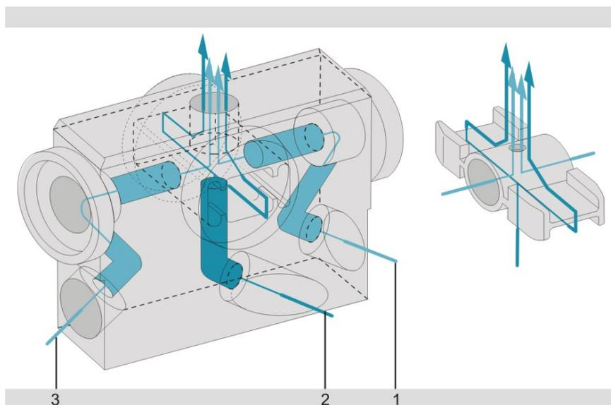
Fig. 14 Primary and outer gas flows in the graphite tube furnace
