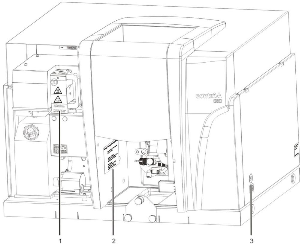
Fig. 2 Warnings and notice signs at the front and side panels
