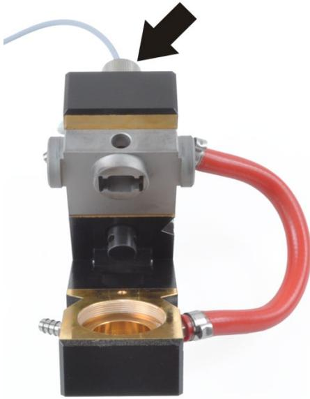
11. Detach the union nut at the cooling water temperature sensor.
