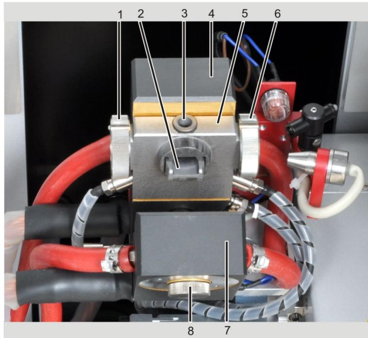
Fig. 36 Open graphite tube furnace with inserted graphite tube
