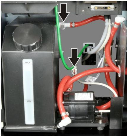
**Reinstalling the cooling water tank assembly:**
