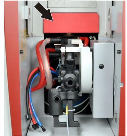
Fig. 62 Installation of the transport lock in the sample chamber
