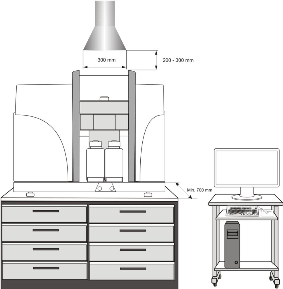
Fig. 6 contrAA 800 workspace with exhaust unit
