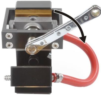
16. Align the furnace jacket with the cylindrical adapter parallel to the furnace body and fasten it with the inserting tool (large bracket).
