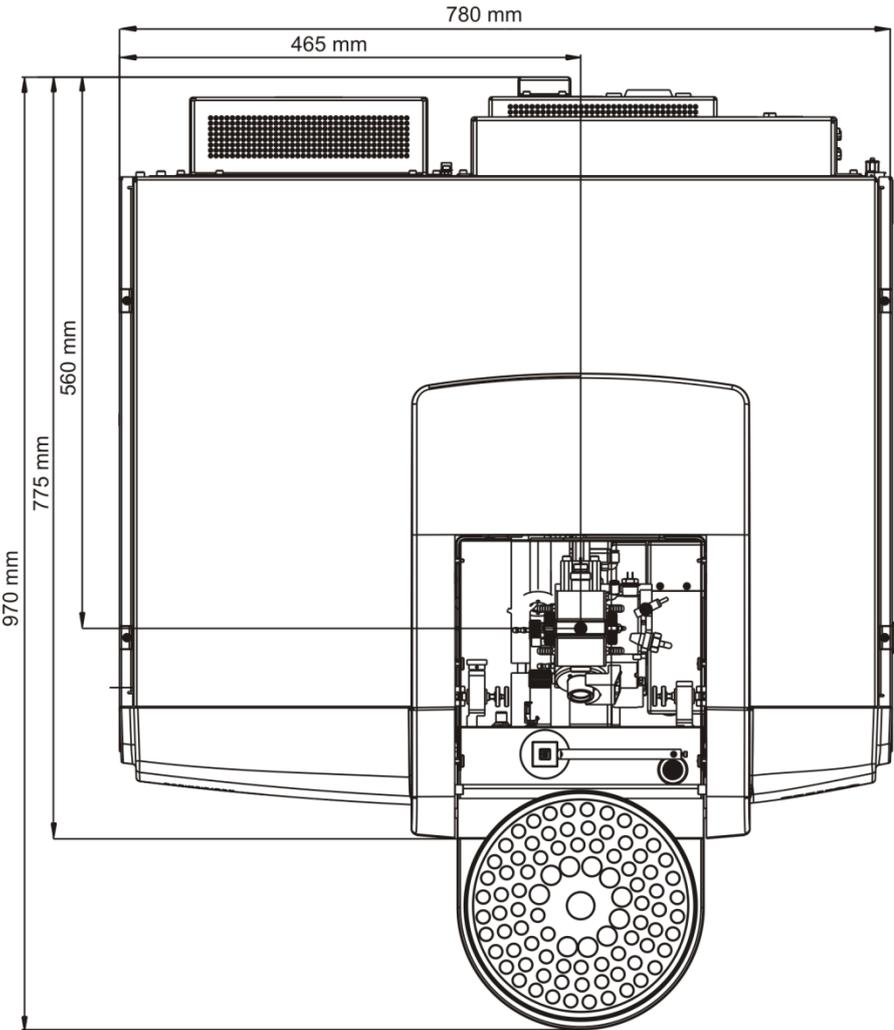
Fig. 3 contrAA 800 dimensions – top view (with autosampler AS-GF)
