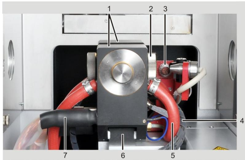
Fig. 34 Connections at the graphite tube furnace
