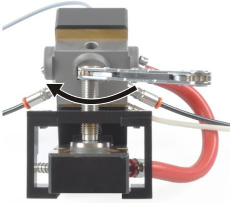
23. Position a new electrode parallel to the movable furnace part and secure it with the inserting tool (small bracket).
