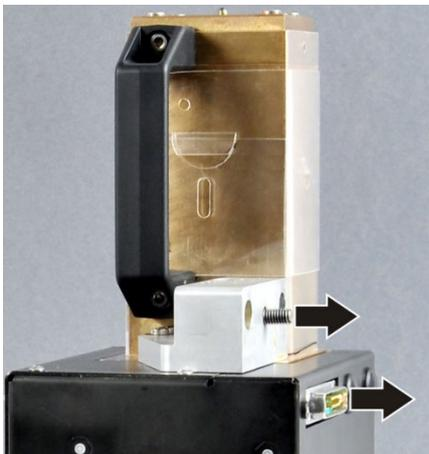
**Reinstalling the lamp housing:**
