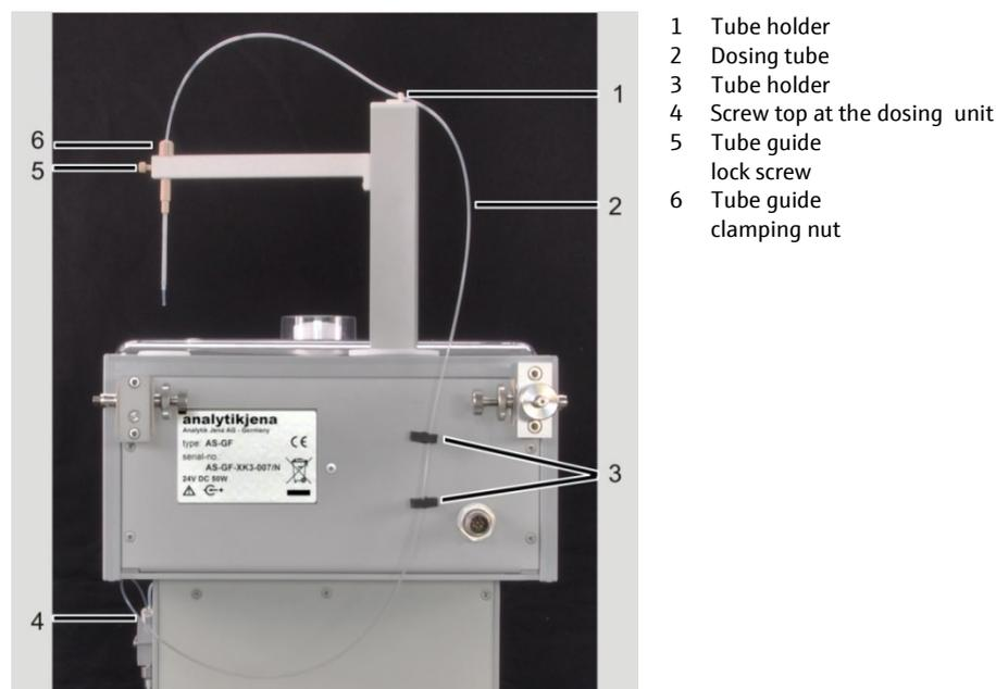
Fig. 60 Dosing tube at the AS-GF
