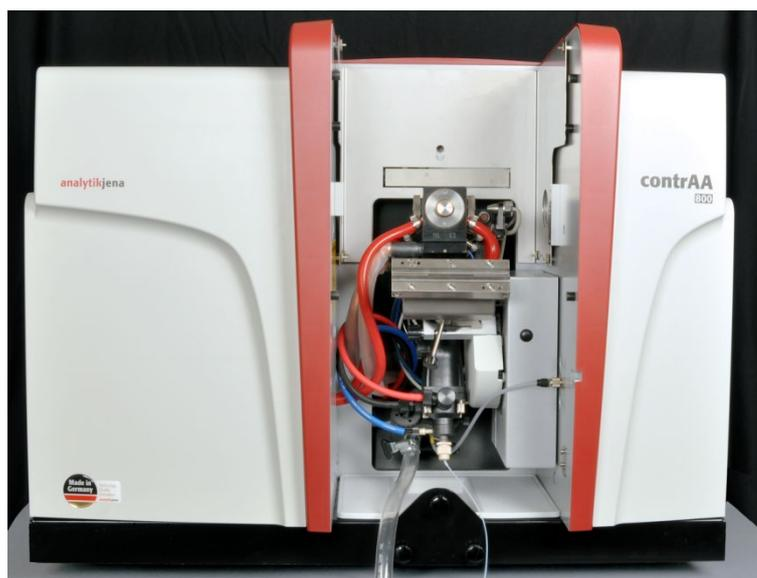
Fig. 8 Sample chamber of the contrAA 800 D
