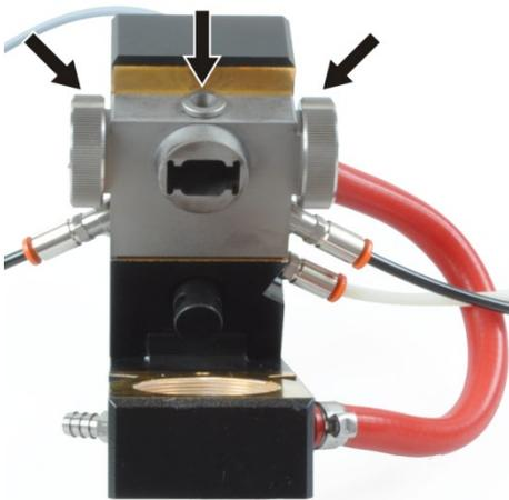
9. Pull the furnace windows off the furnace jacket. Remove the pipetter insert.
