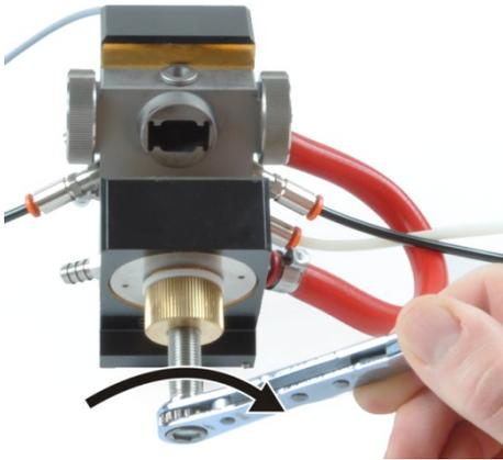
8. Screw the press-out tool with the spindle turned back to the stop into the movable furnace part.
