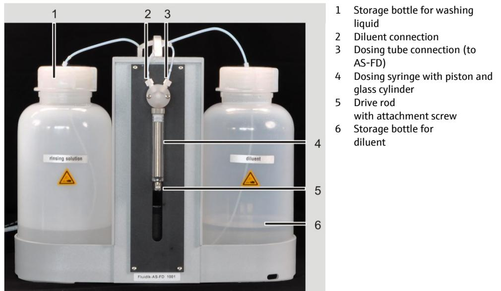
Fig. 45 Dosing unit at the Fluidik module of the AS-FD
