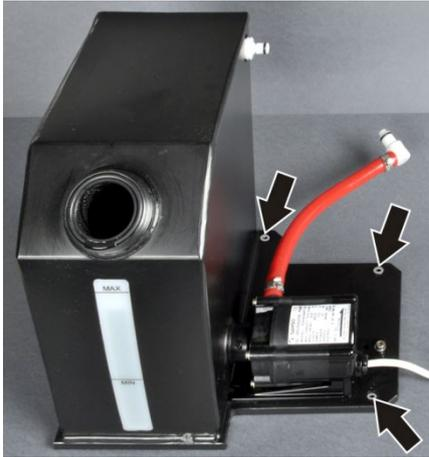
9. Detach the screws securing the assembly (see arrows).
