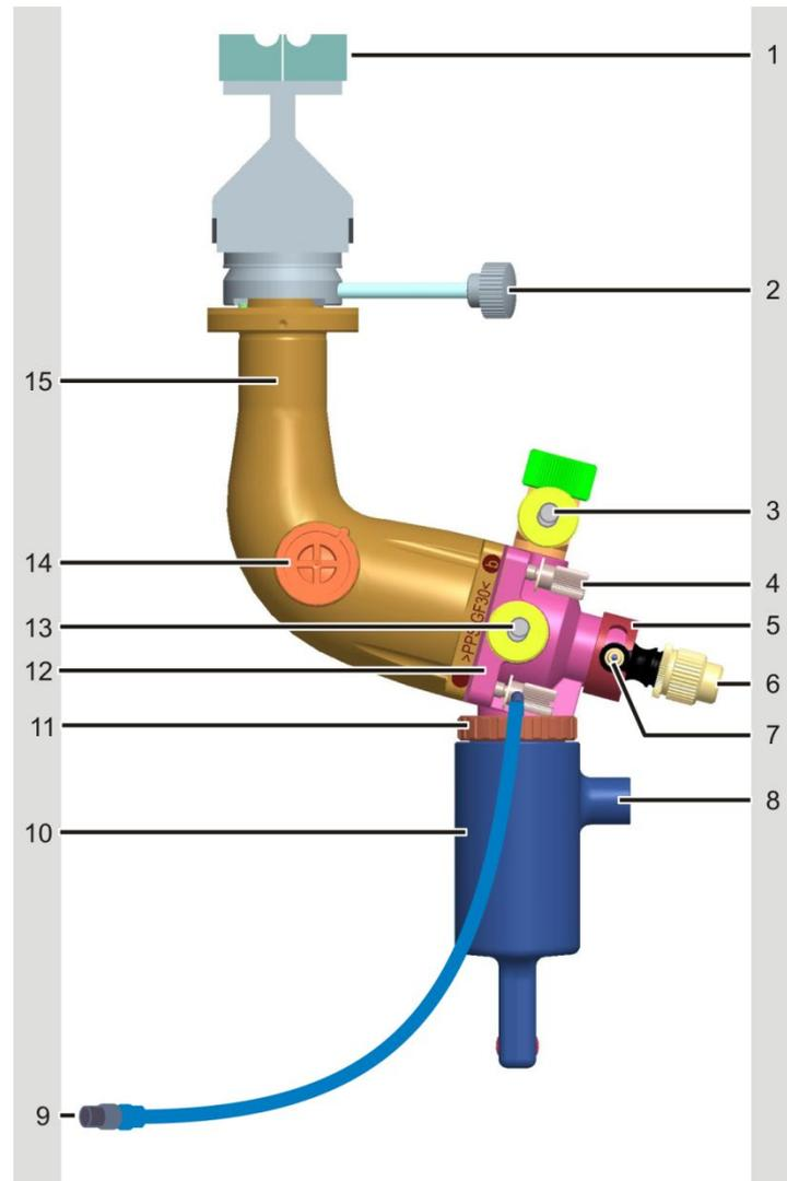
Fig. 20 Nebulizer mixing-chamber burner-system
