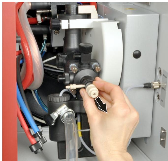
Fig. 56 Withdrawing the nebulizer from the mixing chamber
