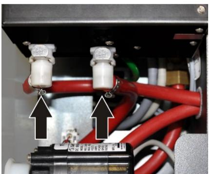
18. Connect the cooling water hoses at the underside of the lamp housing.
