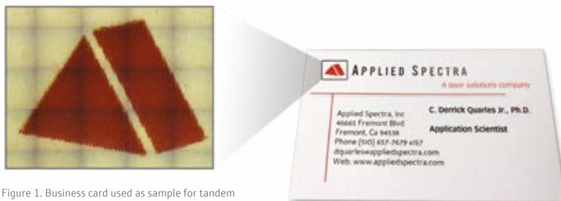
Figure 1. Business card used as sample for tandem LA-ICP-MS & LIBS analysis.
