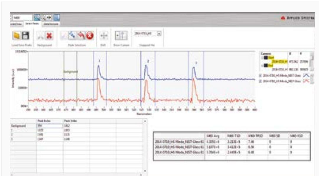
Figure 2. ASI LA data analysis software screen shot illustrating how transient data can be integrated. Any ICP-MS data files can be loaded into the data analysis program, allowing the J200 LA instrument to be coupled with any ICP-MS instruments. An example of the integrated data is displayed for 60Ni in the bottom right of the screen shot (All elements are integrated and saved into the data file, but 60Ni shown above for simplicity).
