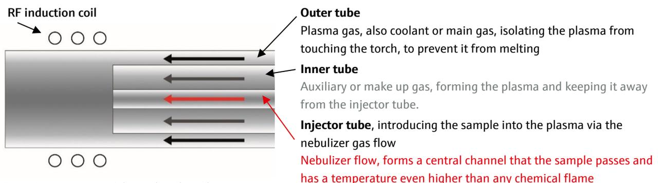
Figure 1: construction of the torch and gas flows
