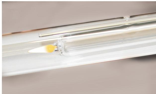
Figure 2: Multi-purpose combustion tube with optical fiber
