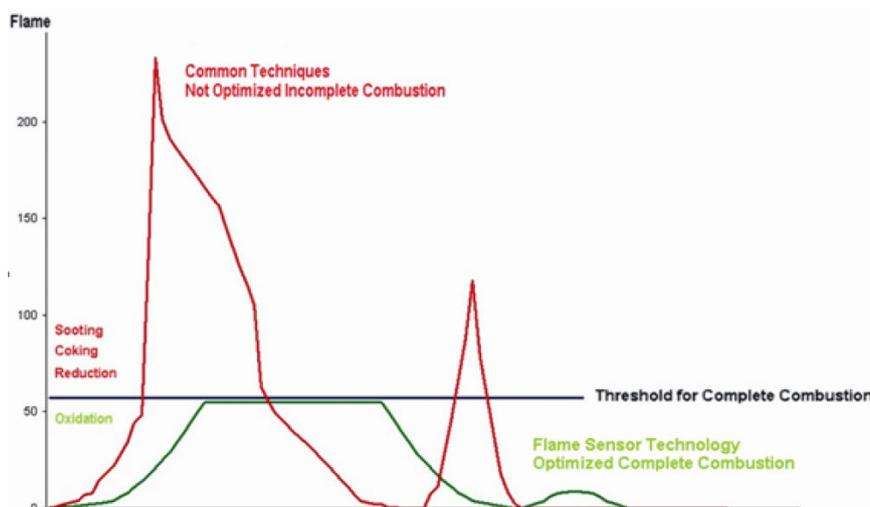
Figure 3: Optimized digestion process with flame sensor technology
