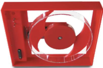
Rotaphor rotor with computer controlled electrodes and connection plug. Electrodes are freely rotatable, thus providing a maximum of flexibility.
