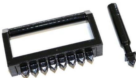
Reagent Plates or Strips are prefilled with extraction reagents and are sealed with a foil. Prior to use this foil has to be pierced manually, by using the piercing tools (single piercer or 8fold piercer).
