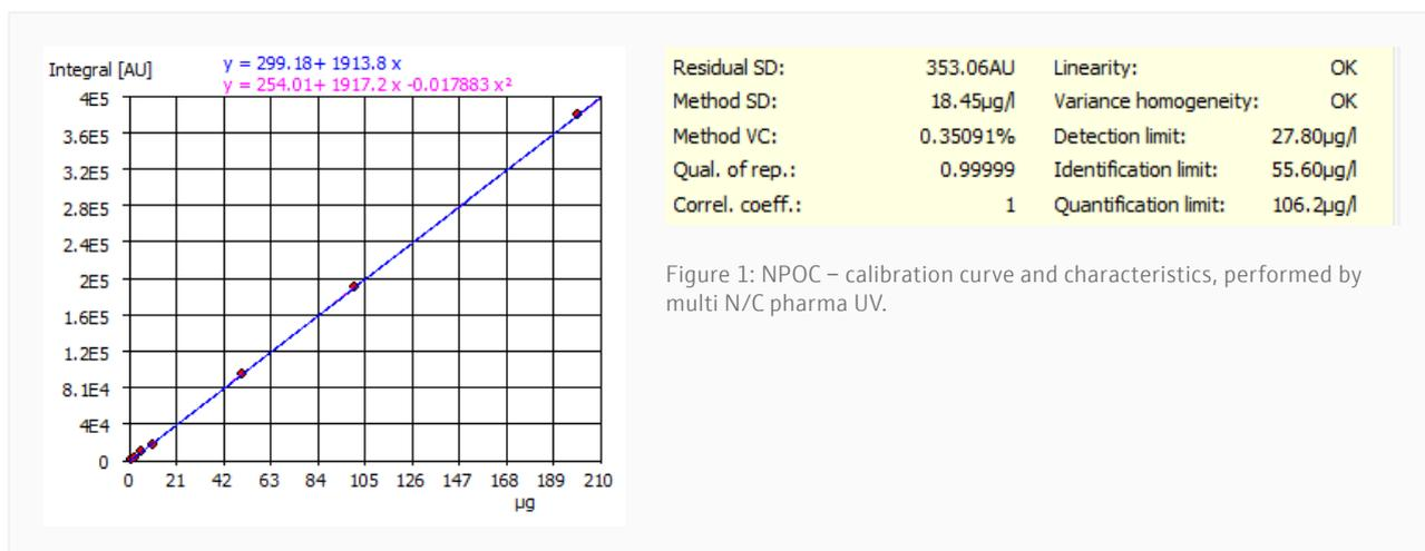
Figure 1: NPOC – calibration curve and characteristics, performed by multi N/C pharma UV.
