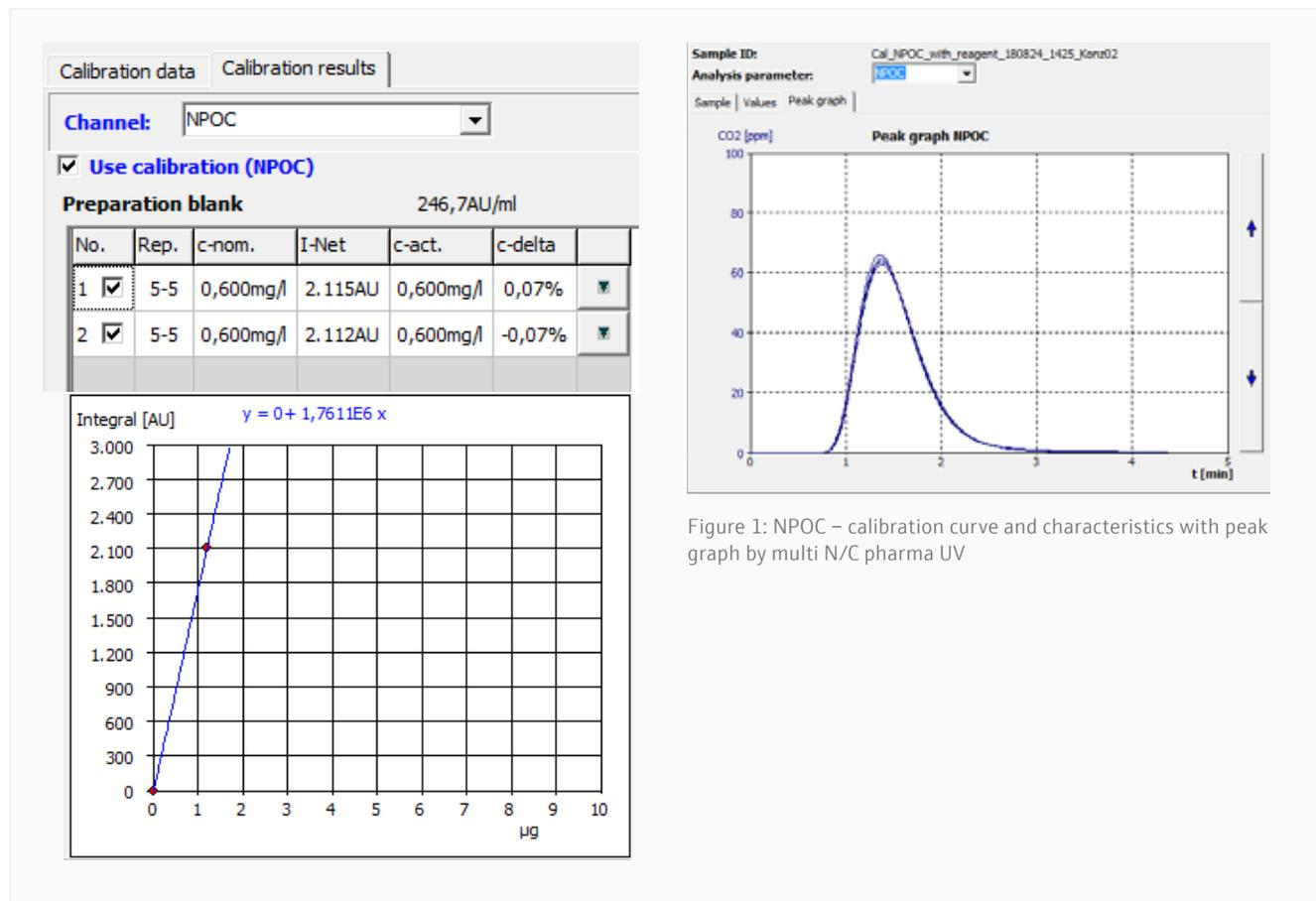
Figure 1: NPOC – calibration curve and characteristics with peak graph by multi N/C pharma UV
