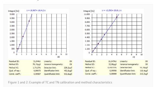
Within the method up to three calibration ranges can be linked to each parameter in order to cover an over-all working range of up to three magnitudes. With the NPOC/TN $_{\rm b}$  method three NPOC and two TN $_{\rm b}$  multi-point calibration ranges were linked as follows:
